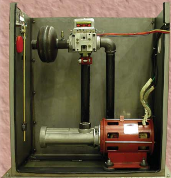
Hydraulic Power Units
